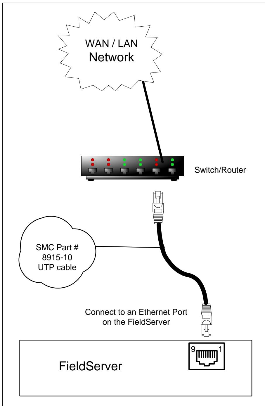
The Ethernet connection can be achieved using a switch or crossover cable. The driver will support all Ethernet connections on a local area network (LAN) or wide area network (WAN) including internet connections and crossover cable connections.
